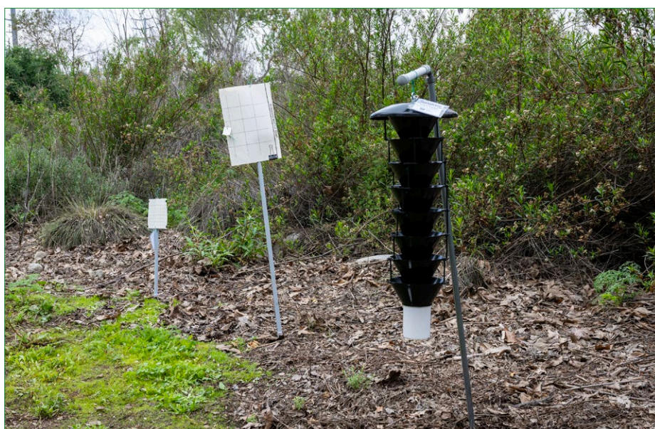
Figure 7: Sticky panel trap set up on a pole (left) and Lindgren funnel trap (right).
