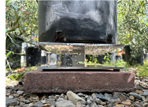
Figure 4. Load Cell measuring weight and daily water use of an Olive tree planted in a 15-gal container.
