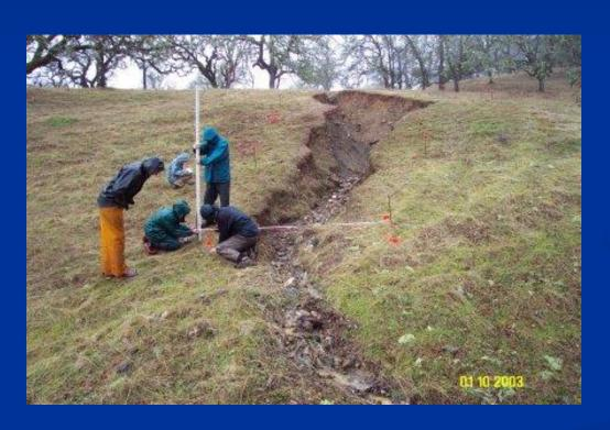
Both of these gullies originated at points of road drainage discharge
