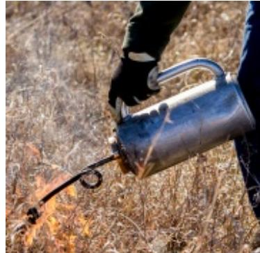
A drip torch probably is the most useful and widely used ignition tool on prescribed burns. Drip torch fuel typically is a mixture gasoline and diesel with 20-50 percent gasoline depending upon air temperature and fuel conditions. Additional pre-mixed drip torch fuel generally is brought to a burn in spark and rupture-resistant containers, which allows drip torches to be quickly refilled.
