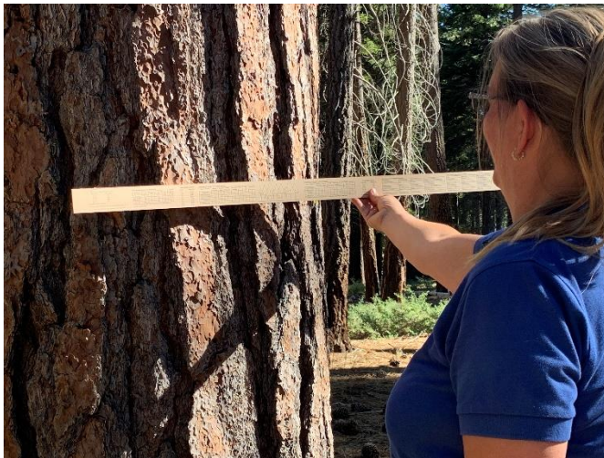
Above: Susie Kocher using a fiberglass reel tape to measure out a plot. Left: using a Biltmore stick to measure diameter at breast height (dbh).
