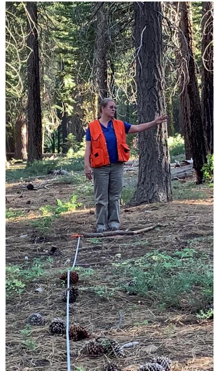
Above: Susie Kocher using a fiberglass reel tape to measure out a plot. Left: using a Biltmore stick to measure diameter at breast height (dbh).
