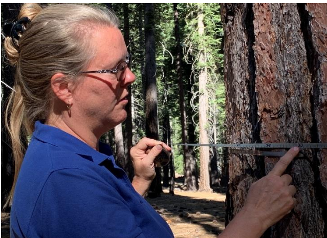
Susie Kocher measuring the diameter of a tree with a diameter tape (or d-tape).
