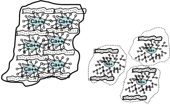
**Figure 14a.** Conceptual illustration of soil aggregate stability: forming stable aggregates with plentiful calcium on clay exchange sites (left), compared to weak soil aggregates due to low salinity and/or excessive sodium in the soil pore water.
