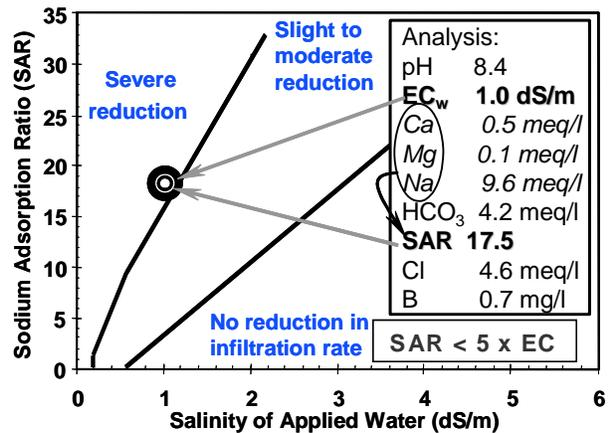
**Figure 14e.** Estimating potential infiltration problems and determining amendment options from an irrigation water analysis.
