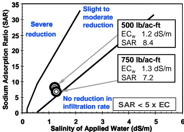
**Figure 14f.** Revised infiltration potential after gypsum amendment to irrigation water for 500 and 750 lb/ac-ft injection rates.
