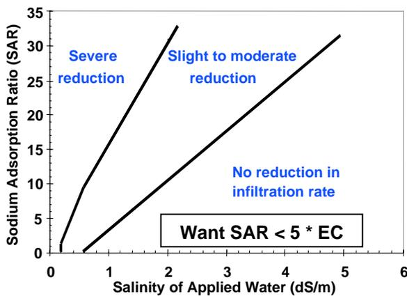
**Figure 14d.** Interaction of total salinity as EC with the sodium adsorption ratio of applied water for causing potential infiltration problems. (Ayers and Westcott., 1985)
