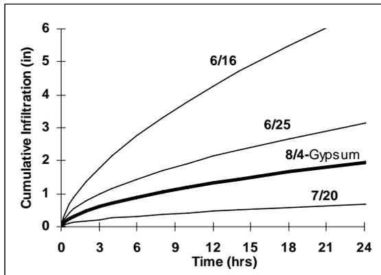
**Figure 14b.** Cumulative depth of infiltration for Wasco sandy loam over the season for the same furrows in furrow irrigated cotton at the Shafter Field Station (Shafter, CA 1995) with low salinity canal water (0.02 dS/m).
