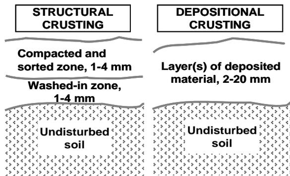
**Figure 14c.** Conceptual illustration of structural and depositional crusts.
