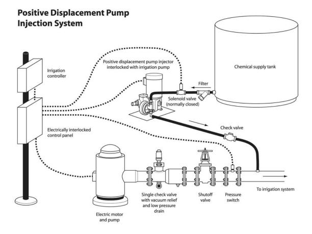
Figure 17c. Typical layout of chemigation injection system.
