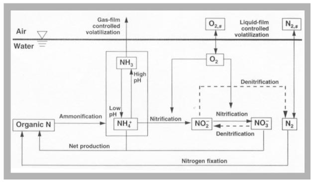
Figure 1. The nitrogen cycle.
