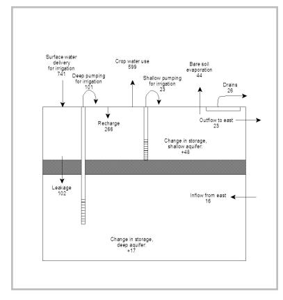
Figure 16: Water balance for a groundwater basin on the west side of the San Joaquin Valley, California. (Modified from Belitz and Phillips, 1995)
