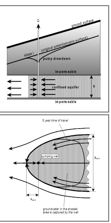
Figure 13: Flow to a well in a uniformly sloping potentiometric surface: (a) cross-section (upper), and (b) plan view (lower). (Modified from EPA, 1994, Figure 4-10)
