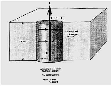
Figure 3: Delineation of wellhead protection area by cylinder method. (From EPA, 1994, Figure 4-4)
