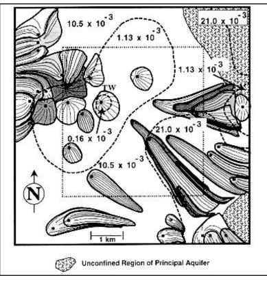
Figure 10: Fifteen-year TOT zones (shapes with flow lines) in a confined aquifer with a complex flow field. Contour lines delineate areas of varying hydraulic conductivities. (From Forster, C. B., T. E. Lachmar, D. S. Oliver, 1997)
