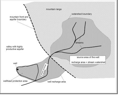
Figure 1: Conceptual illustration showing the relationship of wellhead protection area, recharge area, and source area of a well.
