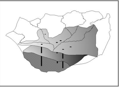
Figure 9: When the aquifer geometry is complex and multiple pumping wells are located near each other, numerical computer modeling may be the best tool for delineating groundwater protection zones.
