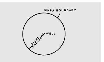
Figure 2: Delineation of wellhead protection area by fixed radius method. (From EPA, 1994, Figure 4-4)
