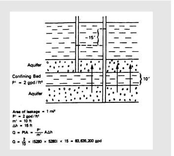
Figure 4: Using Darcy's law to calculate the quantity of leakage from one aquifer to another. (From EPA, 1994, Figure 4-9)
