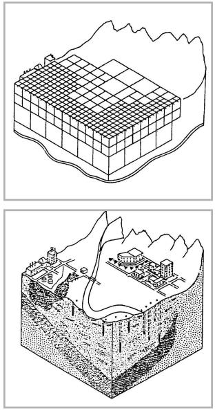
Figure 17: (a) Three-dimensional grid to model groundwater flow in (b) complex geologic settings with pumping wells downgradient from potential contaminant sources. (From EPA, 1994, Figure 6-1)
