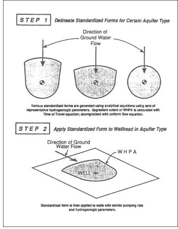
Figure 7: Delineation of wellhead protection area by simplified shapes method. (From EPA, 1994, Figure 4-4)
