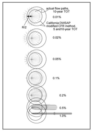
Figure 6: Same as Figure 5, but here the circles indicate the protection zones obtained from the California DWSAP modified CFR method. The CFR method works best at some low to intermediate groundwater level gradients (may vary by aquifer properties). At higher gradients it still provides a poor approximation of the protection zone actually needed.
