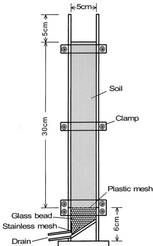
**Fig. 1. Schematic diagram of the soil column.**
