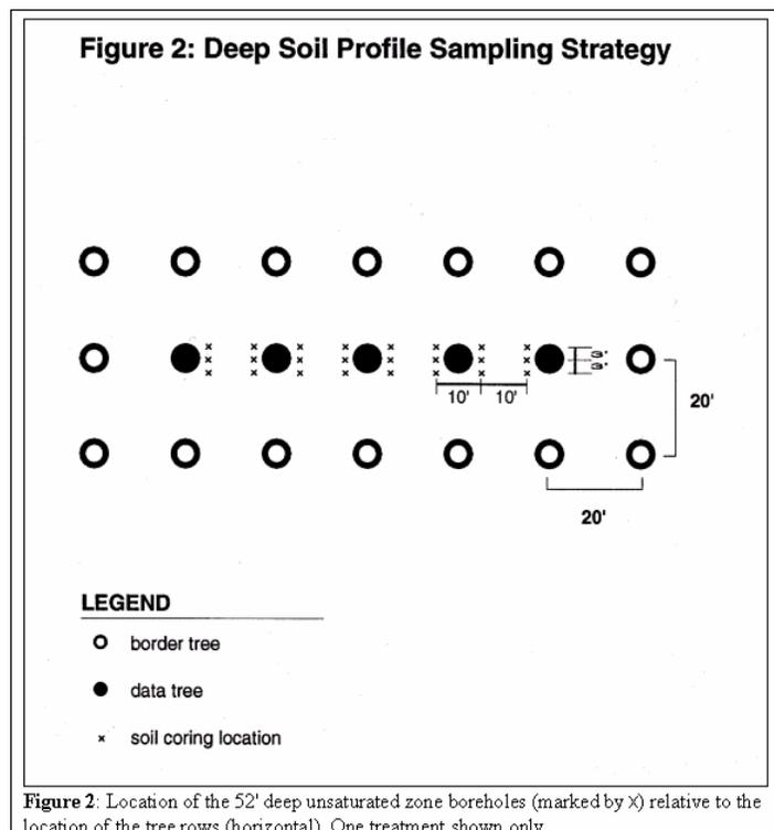
Figure 2: Location of the 52' deep unsaturated zone boreholes (marked by x) relative to the location of the tree rows (horizontal). One treatment shown only.
