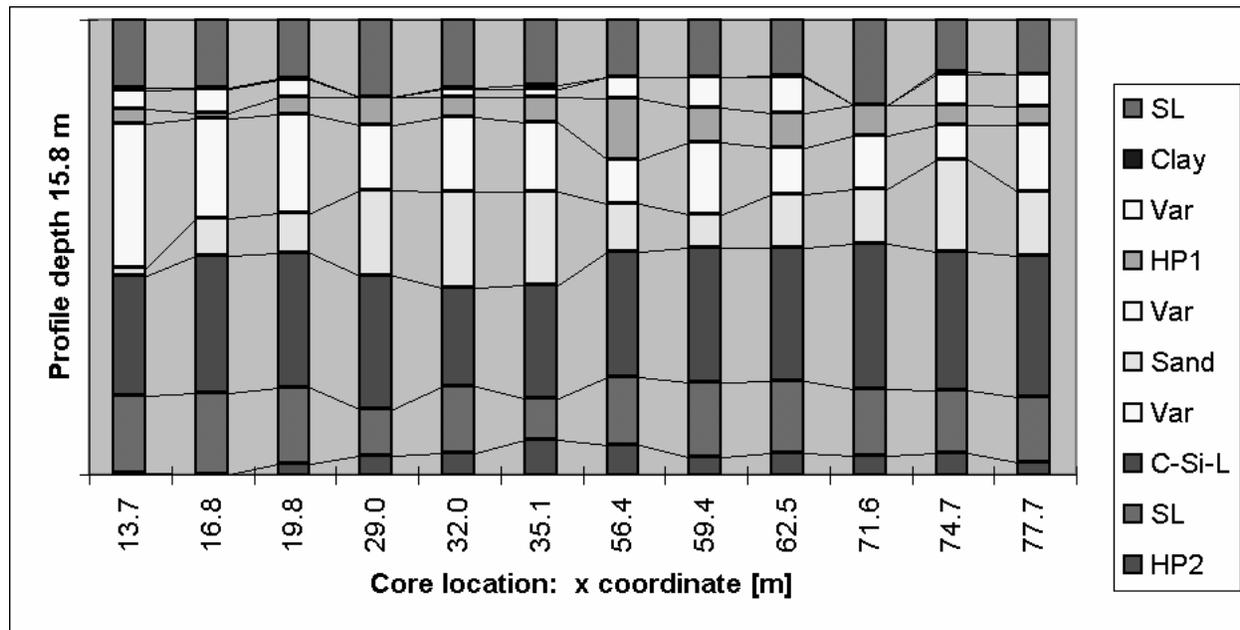
**Figure 3:** Stratigraphic cross-section along a tree-row showing the major stratigraphic units.
