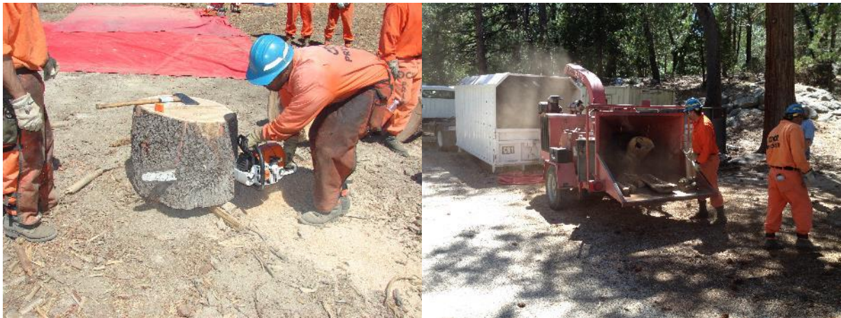
Slabbing and Chipping of GSOB-infested oak rounds (unchipped slabs were used as controls)
