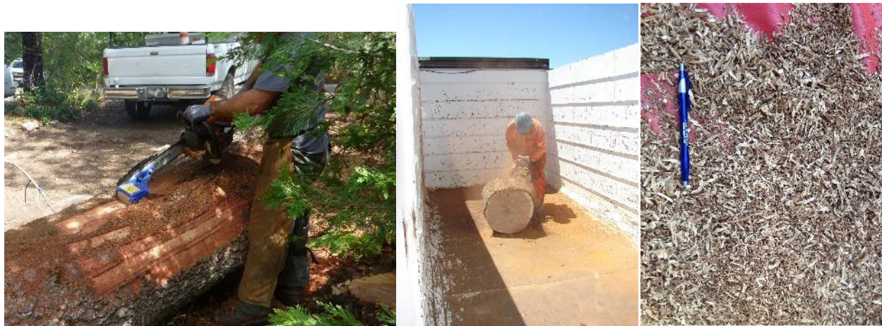
The chainsaw-powered debarkers produced very fine bark chips.
