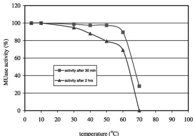
Fig. 3. Temperature stability of MUase activity. For temperature stability tests enzyme in 25 mM buffer was incubated at 4–70 °C for times specified in graph. Prior to the assay at 30 °C, the enzyme mixture was brought back to room temperature. Numbers represent the mean of three replicates with a CV < 11%.
