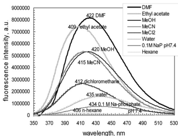
**Fig. (7).** Solvent effects on fluorescence spectra of XIIa (excitation 300 nm). Numbers in front of the solvent show the emission maximum.
