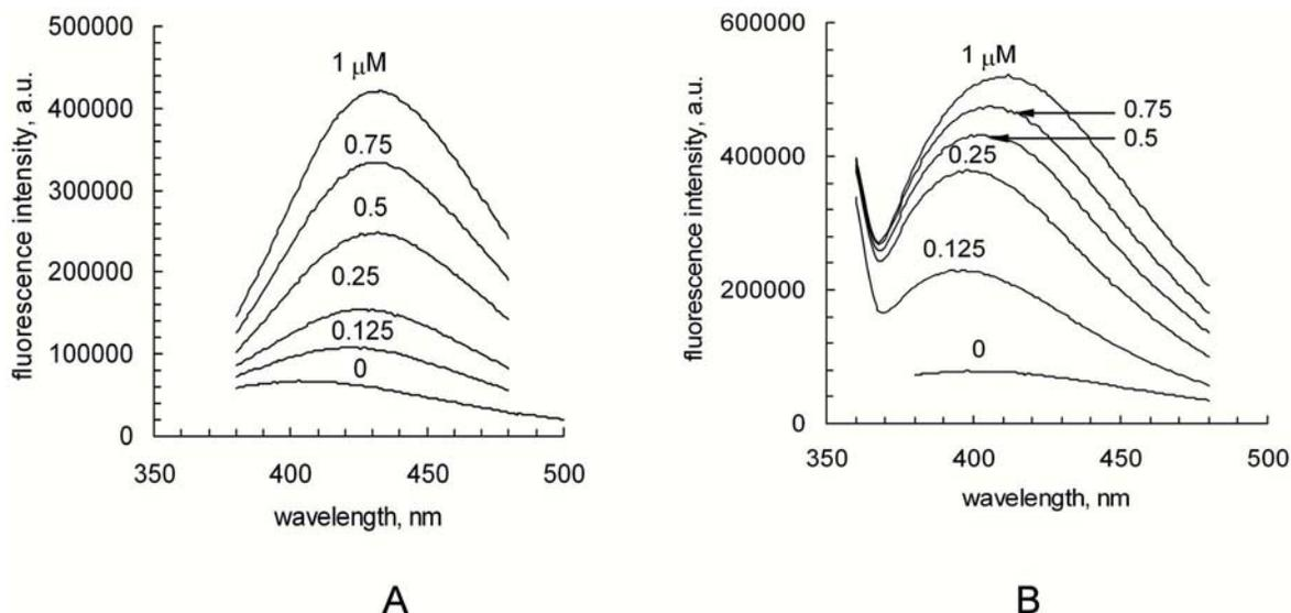
**Fig. (3).** Fluorescence spectra of XIIa (at excitation 330 nm) in absence (A) and in the presence (B) of 50 nM EH; [XIIa] varies from 0 to 1 μM.
