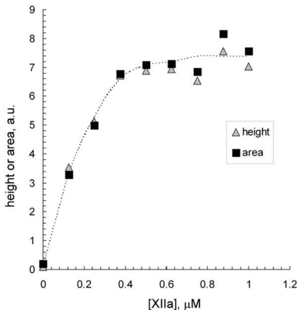
**Fig. (6).** Height and area (according to the Lorentzian fitting) of the 392-nm fluorescence peak of the mixture EH + XIIa at varied concentrations of XIIa ([EH] = 50 nM).
