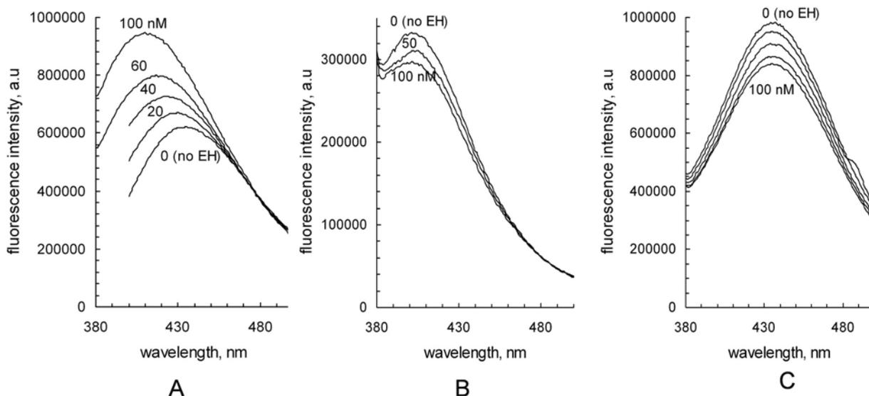
**Fig. (2).** Fluorescence spectra of XIIa (A), XIIb (B), and XIIc (C) (excited at 330 nm) in the presence of varied concentrations of EH (0-100 nM). C: EH = 0, 20, 40, 60, and 100 nM.
