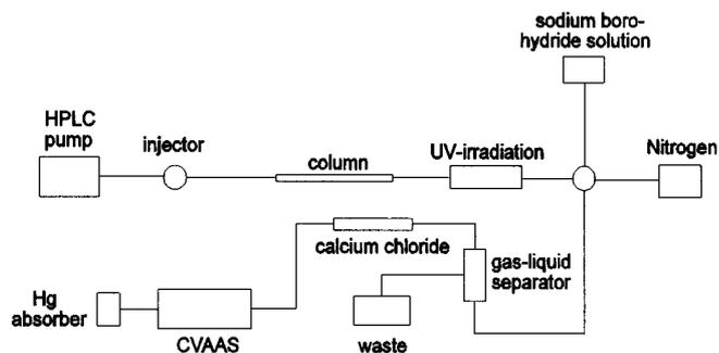
**Fig. 1** Schematic diagram of the HPLC-UV-PCO-CVAAS system coupled with on-line UV-irradiation and continuous-flow mercury generation for the determination of methylmercury and inorganic mercury
