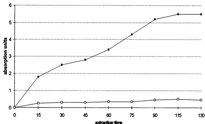
**Fig. 2** Increasing of the detectable  $\text{Hg}^{2+}$  and  $\text{CH}_3\text{Hg}^+$  during the extraction procedure. Extraction conditions: a 600 mg hair sample was extracted by 5 ml of the pyrrolidinedithiocarbamate solution, injecting 20  $\mu$ l at 15 min intervals, respectively
