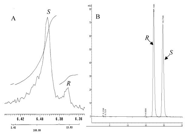
**Figure 3.** (A) <sup>1</sup>H NMR spectrum (Mercury 300 Hz) of cyanohydrin derivative with (1R,2S,5R)-(-)-menthylchloroformate showing the two peaks of the methine proton  $\alpha$  to the cyanohydrin group. (B) HPLC chiral chromatography of *R/S*-acetate with the following conditions: CHIRALCEL, OD-H column (4.6 mm × 250 mm, 5  $\mu$ m particle size); mobile phase, 2.5% 2-propanol in hexane at room temperature; and maximal absorbance, 235 nm.
