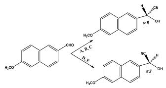
**Figure 4.** Scheme for synthesis of chiral  $\alpha$ -2-hydroxy-2-(6-methoxy-2-naphthyl)acetonitrile. A–E indicate preparation methods described in the Experimental Procedures.
