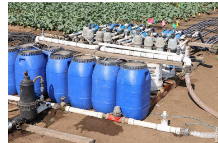
An injection system generated irrigation water with NO 3 -N concentrations of 12, 25 and 45 mg/L.
