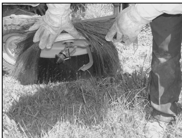
Figure 1. Enviromist sprayer with shield reduces the volume of water and herbicide needed.
