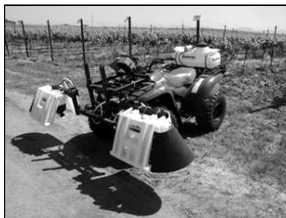
Figure 2. Smart Sprayer; a shielded selective sprayer that treats the weeds, not the bare soil.
