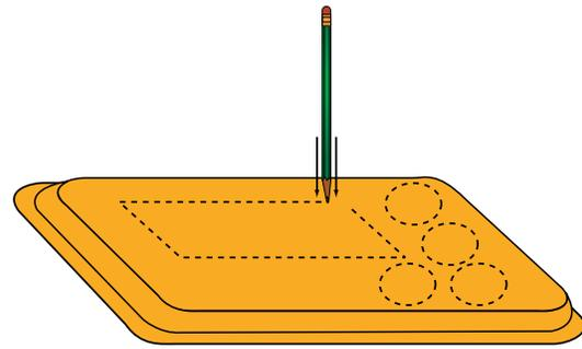
**2.** Punch a small hole in the center of each wheel with the pencil. Push the axle (stirrer) straw through the hole of one wheel so that it extends 1 cm on the other side. Pinch a piece of masking tape around the end of the straw and smooth it on to the wheel. Do the same for the second axle. Do not add wheels to the other ends yet!
