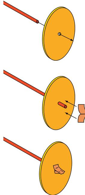
**3.** Cut two large straws to the size you want. Tape them parallel to each other on the bottom of the racer body at opposite ends. Slide a wheel and axle through one of the straws and mount a second wheel on the other end of the axle.
