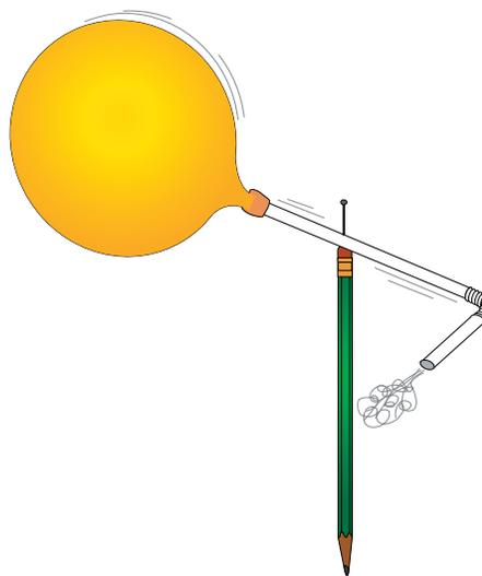
Demonstrate the action-reaction principle by inserting a pin through the straw and into a pencil eraser. Inflate the balloon, and it will pinwheel around the pencil as air rushes out. Compare this to the straight thrust produced by the balloon in the rocket cars.
