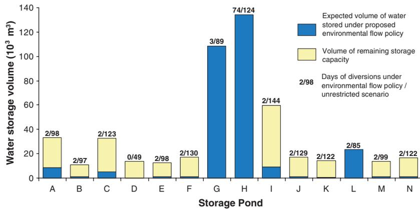
**Fig. 4** Volumes of water stored under an environmental flow policy that restricts period of diversions to allow for fish migrations. Numbers above bars indicate the number of days that water could be diverted from streams to fill ponds under the environmental flow policy and when diversions are unregulated. When winter flow diversions are not restricted, all ponds are filled to capacity.
