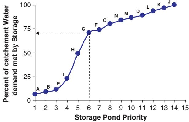
**Fig. 3** Cumulative water storage capacity in catchment by pond priority, based on their benefit-to-impact ratio. Dashed line indicates that approximately 70% of total basin water demand could be met by installing the 6 highest-priority storage ponds.
