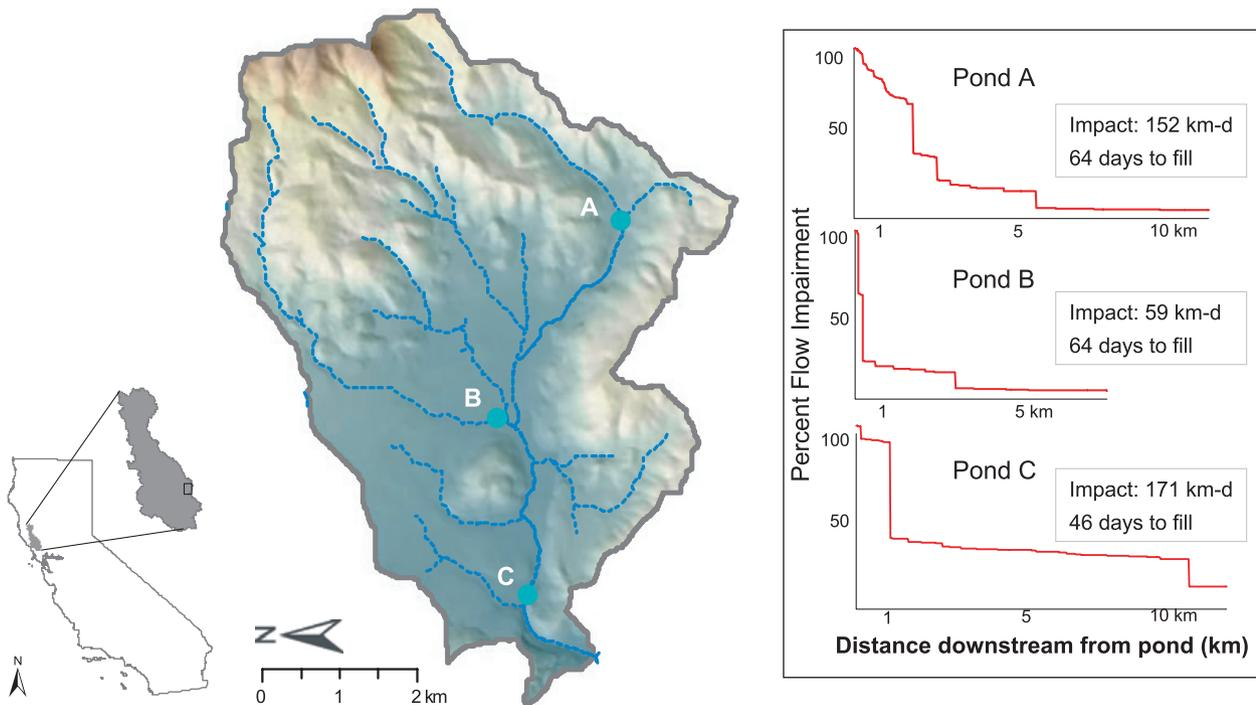
**Fig. 1** Location of three hypothetical agricultural storage ponds (blue circles) of equal volume placed in a subcatchment of the Russian River in northern California, U.S.A. Graphs in right panel show the impact of each pond as percentage of flow impaired with increasing downstream distance from the pond location and report the impact index and time to fill.
