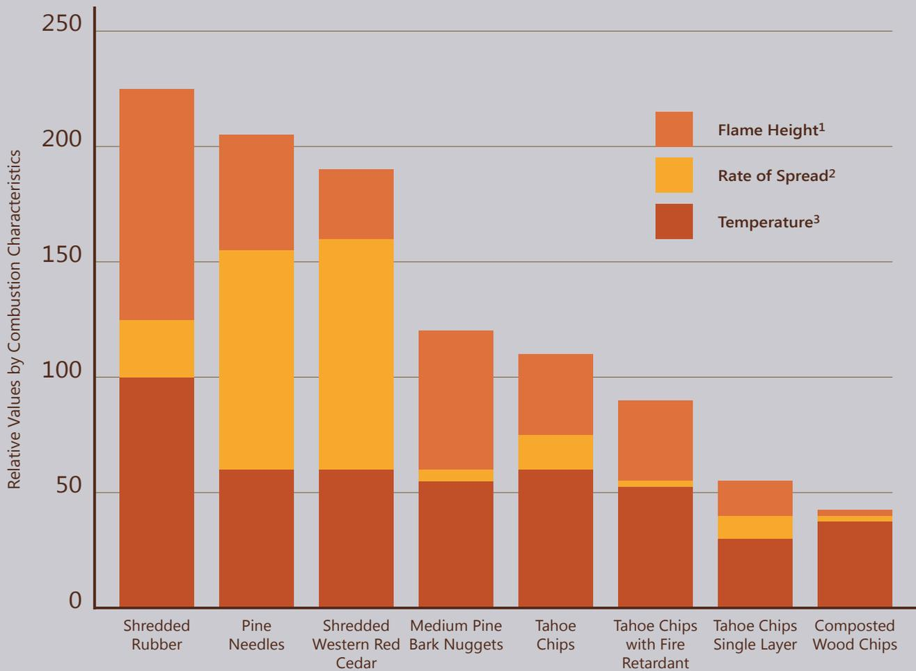
▲ Figure 3. Relative values of three combustion characteristics between eight mulch treatments. <sup>1</sup>Average maximum flame height. <sup>2</sup>Average rate of fire spread. <sup>3</sup>Average maximum temperature measured at four inches above the bed.
