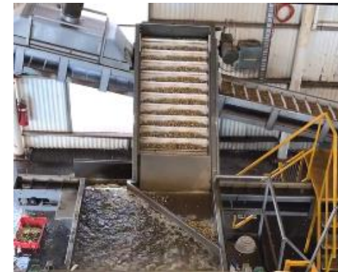
CMV Group: Pistachio float tank
