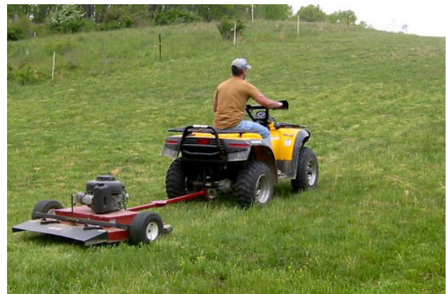
Figure 2. ATV with mower. Operator has shifted weight forward for the hilly operation.
