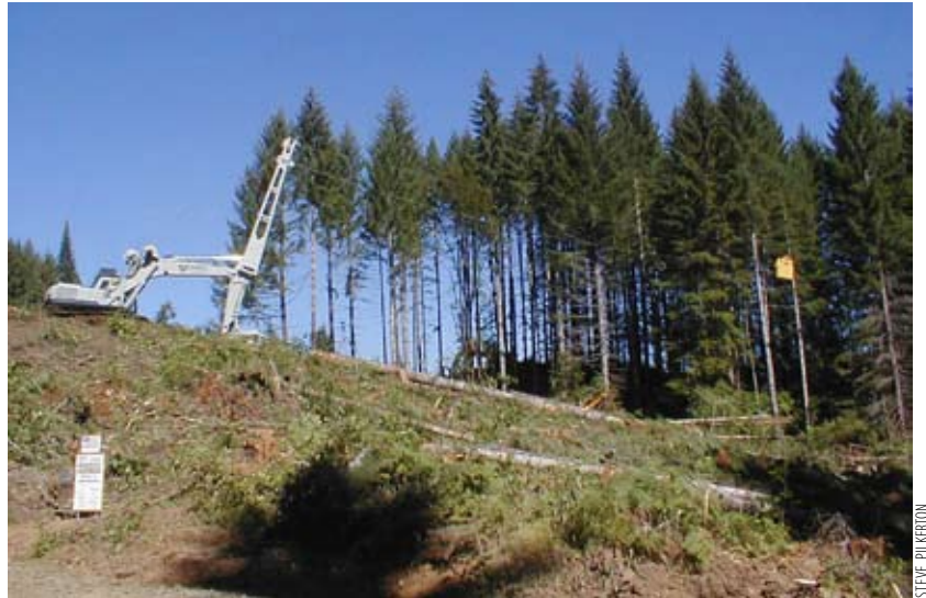
Figure 6.—Cable harvesting on steep ground.
