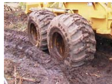
Figure 9.—Soil disturbance from logging with heavy equipment.
