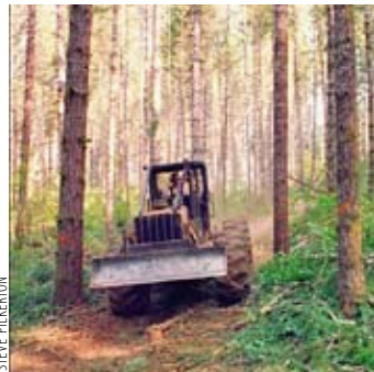
Figure 3.—Harvesting with a rubber-tire skidder.
