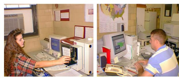
Sample scanned with NIR spectrophotometer
