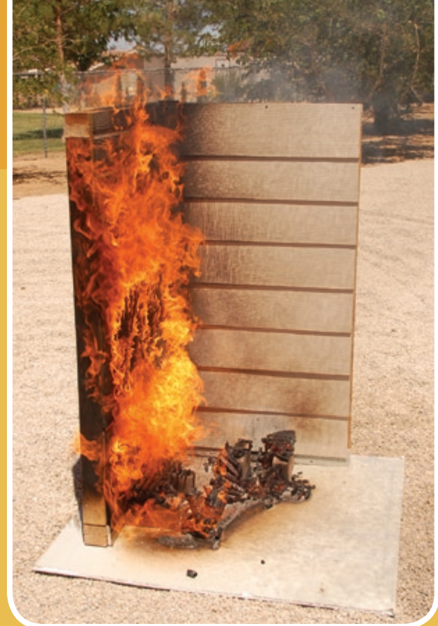
A corner wall section: one side has a composite wood siding product and the other a fiber cement siding product. The ignition source was a burning 'A' brand (12"x12") placed in the corner. It sat on two bricks. This photo was taken ~30 min after the burning 'A' brand was placed in the corner (on the bricks).
