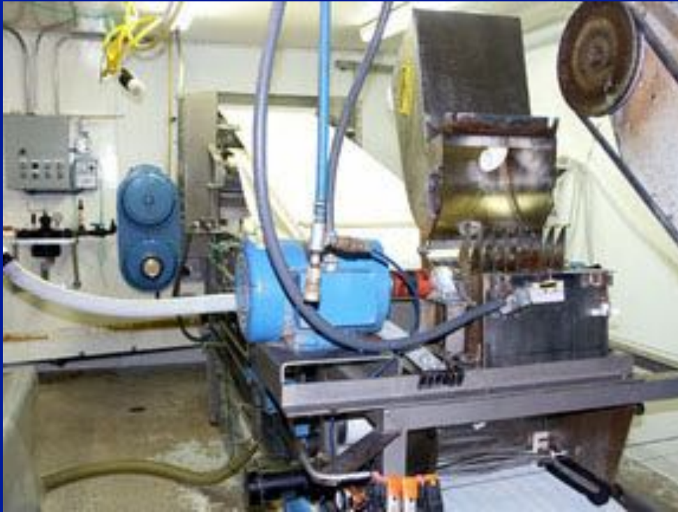
Commercial hammer mill
