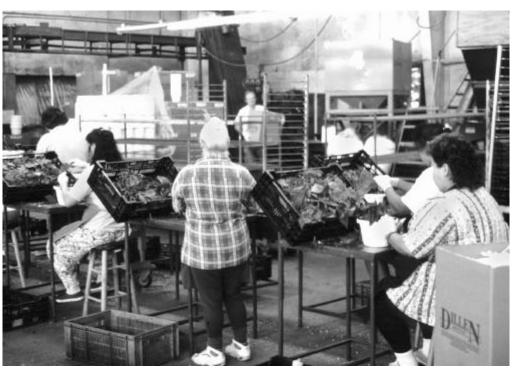
Newly designed stands for potting plants. The stands hold the plant bins at an angle. The slope lets gravity move the plants to the front of the bin so that the plants are always close to the worker and reaching is minimized.
