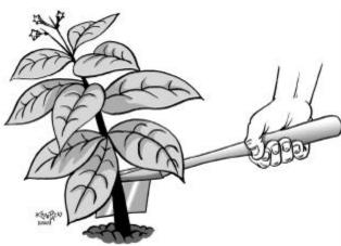
Handle diameter is large enough for small overlap of thumb and fingers.
