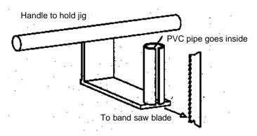
Cut the PVC pipe to 5" lengths and cut an approximately 1/32"-wide slit lengthwise in the PVC using the jig. Use a slotted screwdriver to help slide the PVC over the edge of the tub's existing grip.
