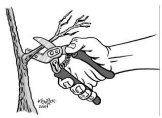
Well-designed tool: Handles are long. Spring return keeps tool open. Handles are covered with rubber or plastic grip.
