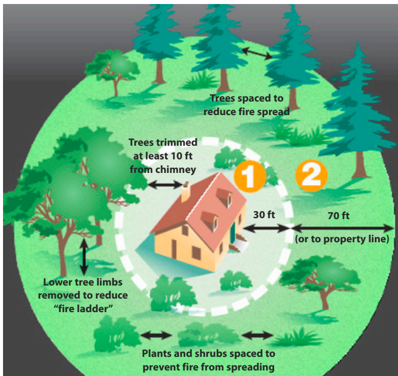
Figure 3. Keep branches trimmed at least 10 feet from your roof and eliminate combustible plants or material under the eaves and next to the house siding and vents. Source: CAL FIRE.
