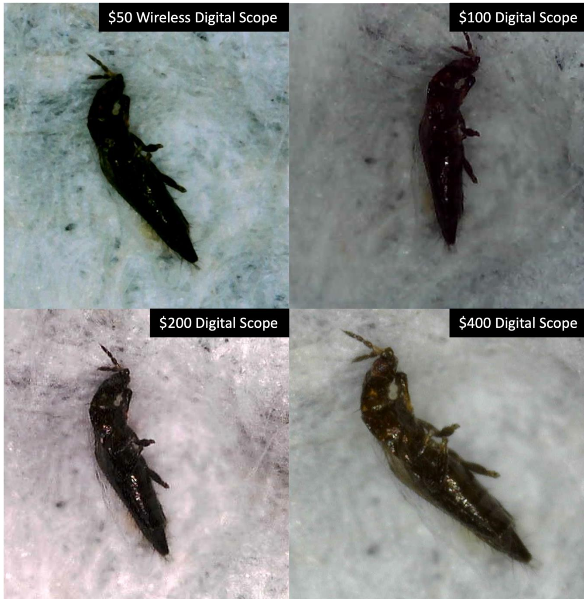
Figure 4. Zooming in on a thrips using variously priced digital scopes. Credit: Eric Middleton, UC IPM.
