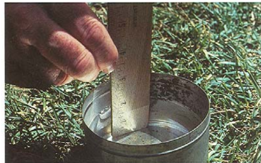
Fig. 2. Measuring depth of water for a "can test."
