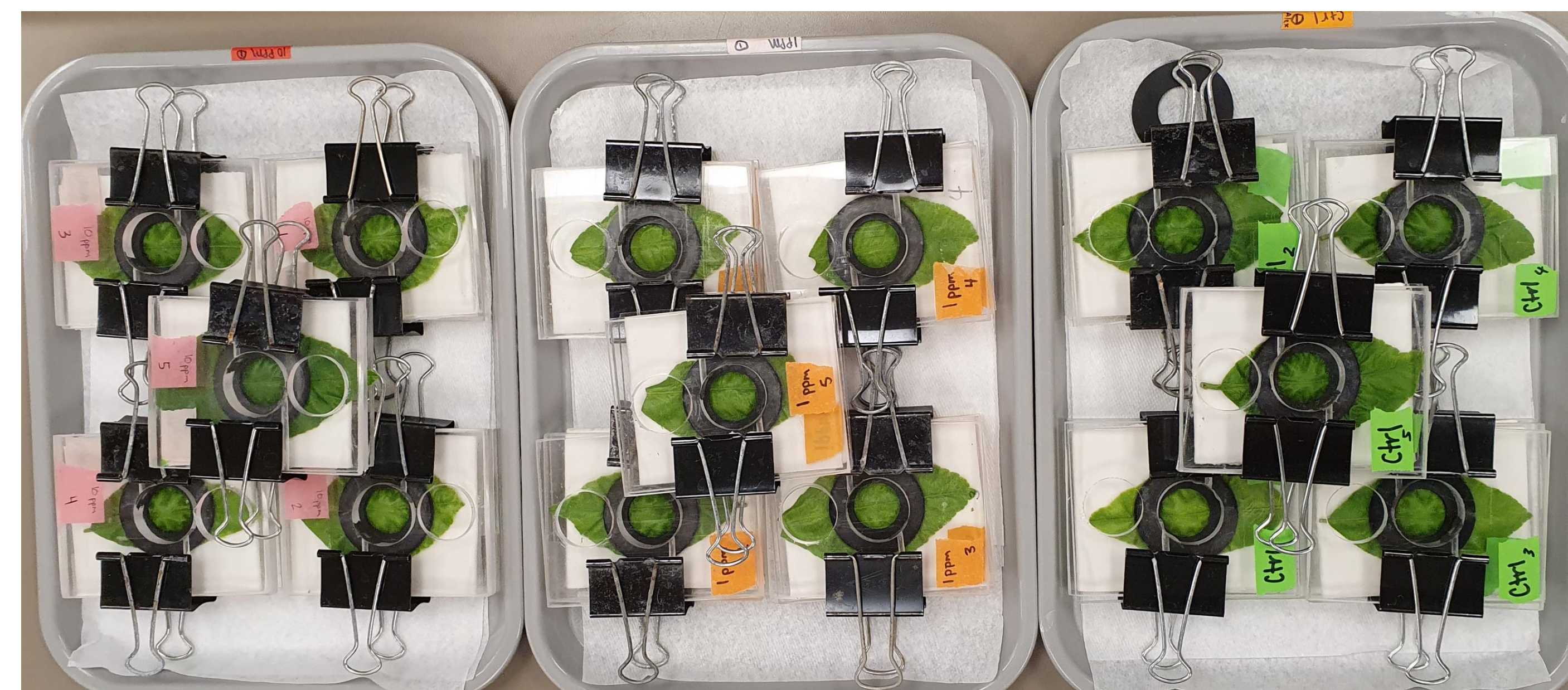
Fig 4. Munger-cell-set for bioassay of citrus thrips resistance to 1 and 10 ppm Delegate along with the control.
