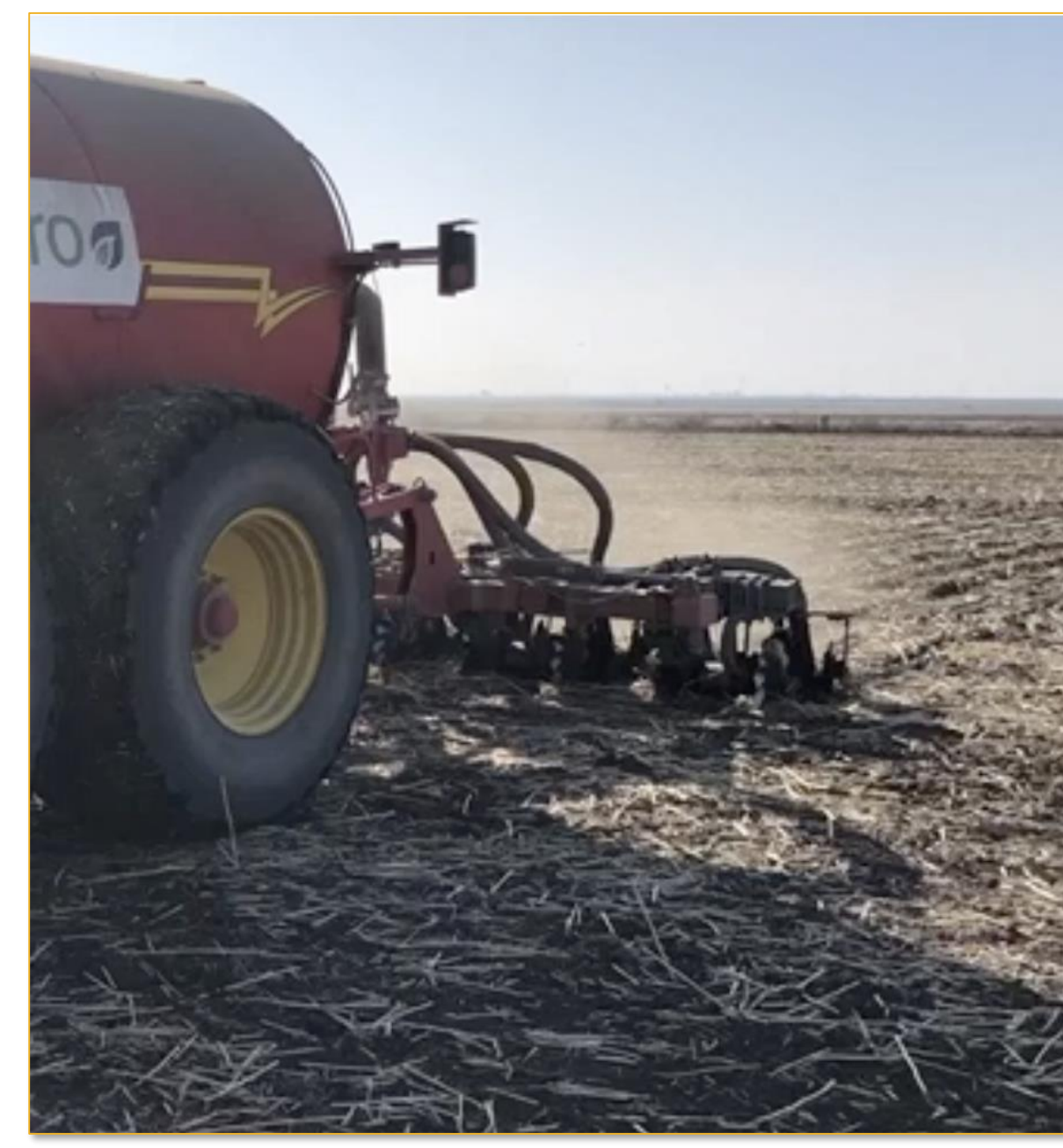
Images: left: Rio Vista, CA where rainfed trials were conducted in 2018. Right: LBF application rig, Coulters open the soil, material is injected, and the soil is closed again by another set of coulters.
