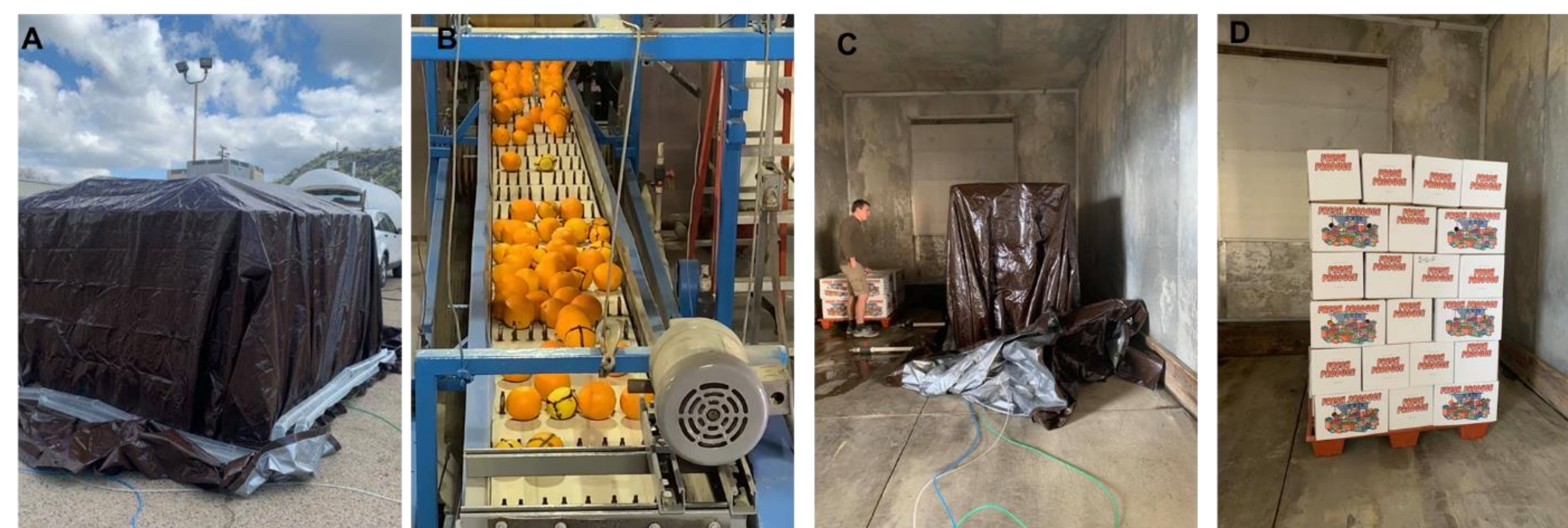
Fig 2. Events of the systems approach; Event 1 (EF)- Vapormate™ fumigation under the tarpaulin (A), Event 2 (Packline) – pressure wash and waxing in the packline (B), Event 3 (PH 3 )- 300-1,000 ppm phosphine fumigation under tarpaulin at 41°F (C), and Event 4 (Cold)- 3-week cold storage at 37°F (D).
