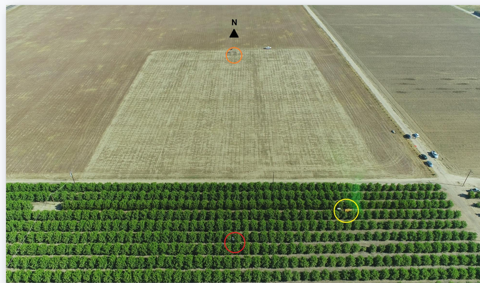
Oblique aerial view of the application area (orchard) and sampling area (light colored area in open field). The sprayer (yellow circle) can be seen moving towards with drifting spray showing as a light green cloud at the rear. The red and orange circles indicate the locations of the weather stations.
