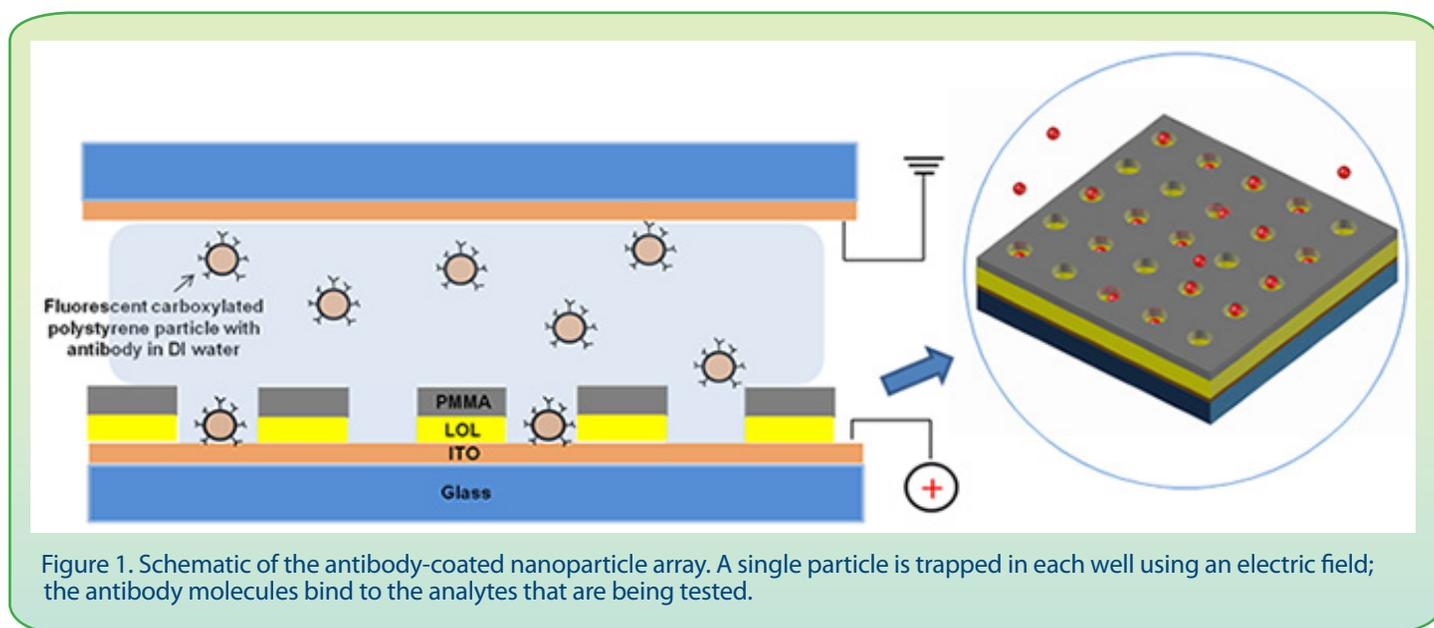
Figure 1. Schematic of the antibody-coated nanoparticle array. A single particle is trapped in each well using an electric field; the antibody molecules bind to the analytes that are being tested.
