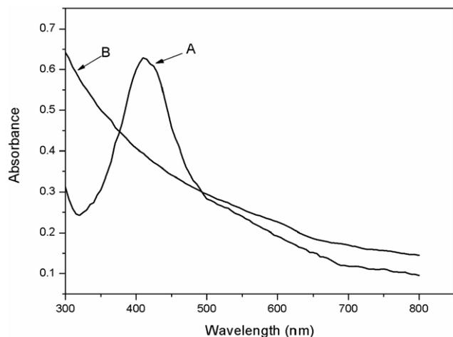
**Figure 4.** Absorption spectra of (A) GLYMO-IDA-doped Ag@SiO<sub>2</sub> nanoparticles and (B) GLYMO-IDA-doped solid SiO<sub>2</sub> nanoparticles without Ag core.
