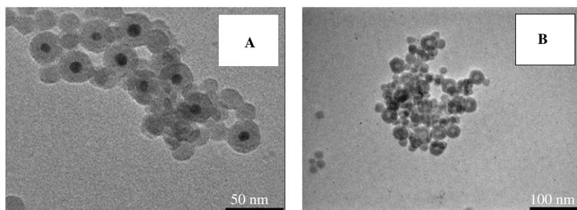
**Figure 3.** TEM images of (A) PDA-doped Ag@SiO<sub>2</sub> nanoparticles, (B) PDA-doped hollow silica nanoparticles without Ag core.
