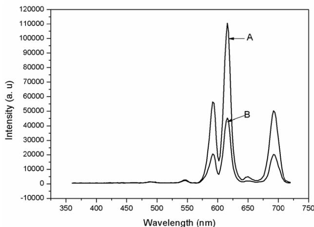
**Figure 5.** Fluorescence emission spectra of (A) Eu<sup>3+</sup>-GLYMO-IDA-doped Ag@SiO<sub>2</sub> nanoparticles, (B) Eu<sup>3+</sup>-GLYMO-IDA-doped solid silica nanoparticles without Ag core.
