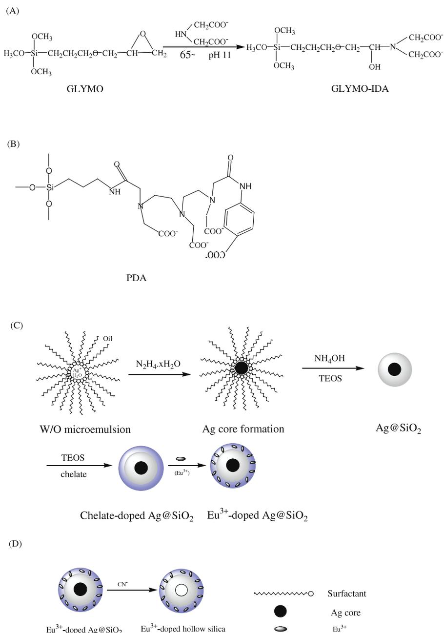
**Figure 1.** Schematic representation of (A) GLYMO-IDA silane; (B) PDA silane; (C) Synthesis of chelate-doped Ag@SiO<sub>2</sub> nanoparticles; (D) Synthesis of hollow SiO<sub>2</sub> nanoparticles.
