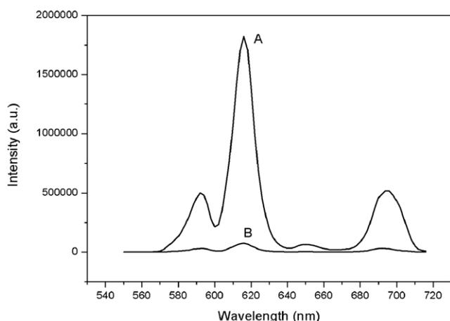
**Figure 7.** Fluorescence emission spectra of (A)  $\text{Eu}^{3+}$ -PDA-doped  $\text{Ag@SiO}_2$  nanoparticles, (B)  $\text{Eu}^{3+}$ -PDA-doped hollow  $\text{SiO}_2$  nanoparticles without Ag core.
