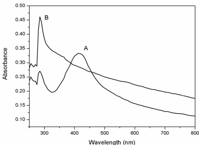
**Figure 6.** Absorption spectra of (A) Eu<sup>3+</sup>-PDA-doped Ag@SiO<sub>2</sub> nanoparticles, (B) Eu<sup>3+</sup>-PDA-doped hollow SiO<sub>2</sub> nanoparticles without Ag core.
