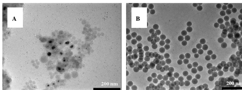
**Figure 2.** TEM images of (A) GLYMO-IDA-doped Ag@SiO<sub>2</sub> nanoparticles, (B) GLYMO-IDA-doped solid SiO<sub>2</sub> nanoparticles without Ag core.
