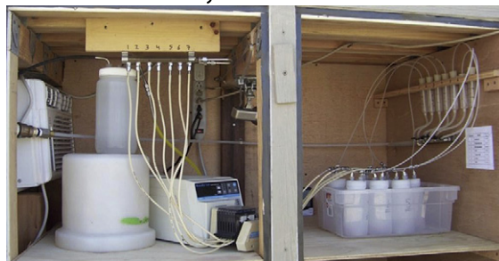
Fig. 2 – Ex situ system set-up: a) schematic of system, illustrating parallel flows through 7 chambers, each containing bio-trap housings with various contents, as listed, b) photo of the interior of the insulated box housing the system, c) schematic of chamber, showing influent and effluent stainless steel lines, each with small slots filed into the inner facing surfaces, and the bio-trap housing centered between influent and effluent lines by bottom fitting and top stainless steel wire (not depicted).
