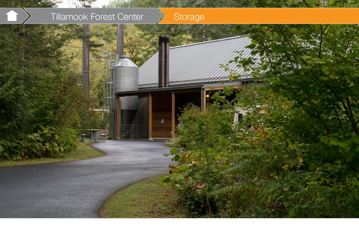
**Storage:** Approximately 64 sq. ft. (8'  $\times$  8') are needed for the 7' diameter, 24' tall, 10-ton grain silo used to store enough pellets to heat the building for a typical winter season. The architects incorporated the agricultural silo into the building's design helping reinforce the theme of a working sawmill.
