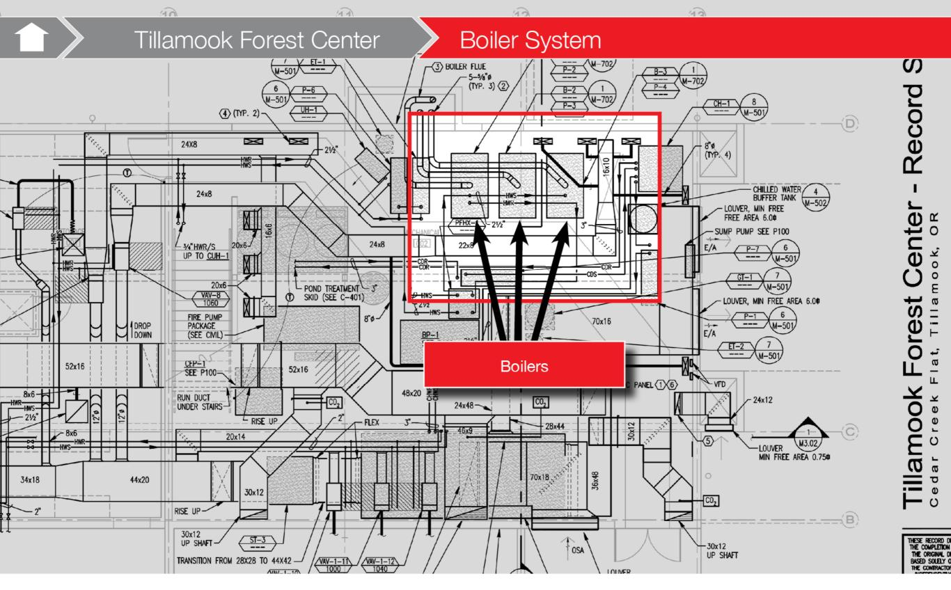
**Boiler System:** The three TARM 136,500 Btu/h wood pellet boilers and related equipment take up about one third of the mechanical equipment room. The rest of the space is used by the air handling system, an air conditioning chiller that uses cool water from a pond in the front of the building, and a fire suppression sprinkler system that also uses treated pond water.
