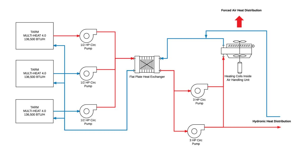
**System Diagram:** Heat is delivered from the boilers to the building using both forced-air (like a furnace in a typical home) and hydronic (hot water loop). A flat plate heat exchanger (center of diagram) is used to isolate the boiler water from the building's hydronic water loop. The three biomass boilers are the only source of heat in the building.
