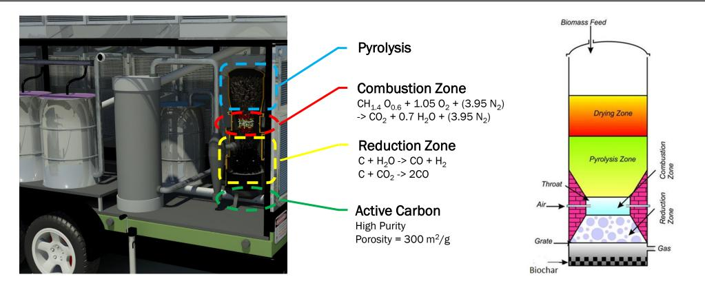
Gasification provides for the best volatile removal from biomass and highest temperature resulting in biochar with extremely high surface area making it usable for multiple applications including animal feed!
