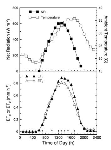
**Fig. 6** The daily time course of Thompson Seedless water use on 7 July 1993 measured with a weighing lysimeter. Values of hourly net radiation (*NR*), ambient temperature (*T*) and reference crop evapotranspiration ( $ET_o$ ) were obtained from the CIMIS weather station at the Kearney Agricultural Center. Net radiation values less than zero were not included. Values of water use ( $ET_c$ ) were expressed on an area basis of 7.55 m<sup>2</sup>. Arrows at the bottom indicate an irrigation event
