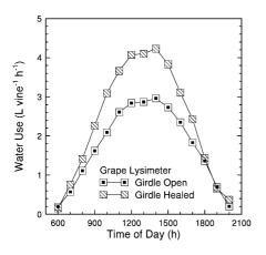
Fig. 4. The daily time course of Thompson Seedless water use measured 3 weeks after the vines were trunk girdled in 1995 (June 27 to July 1 [DOY 178–182]) and once the girdle had healed (callused over) the same year (July 13–17 [DOY 194–198]). Each data point is the mean of hourly values averaged across a 5-day period. Reference ET averaged 6.1 and 5.95 mm day<sup>-1</sup> for the two periods; June 27 to July 1 and July 13–17, respectively.
