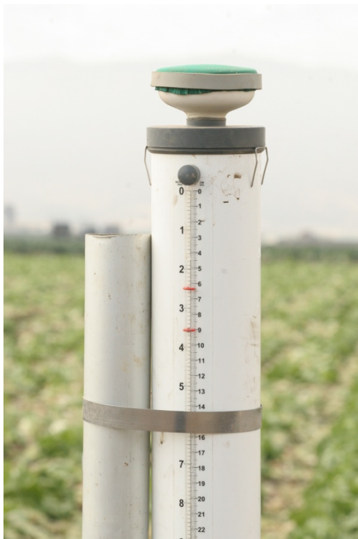
Figure 1. ETgauge® mounted on a post adjacent to a lettuce field. Photo by M. Cahn.
