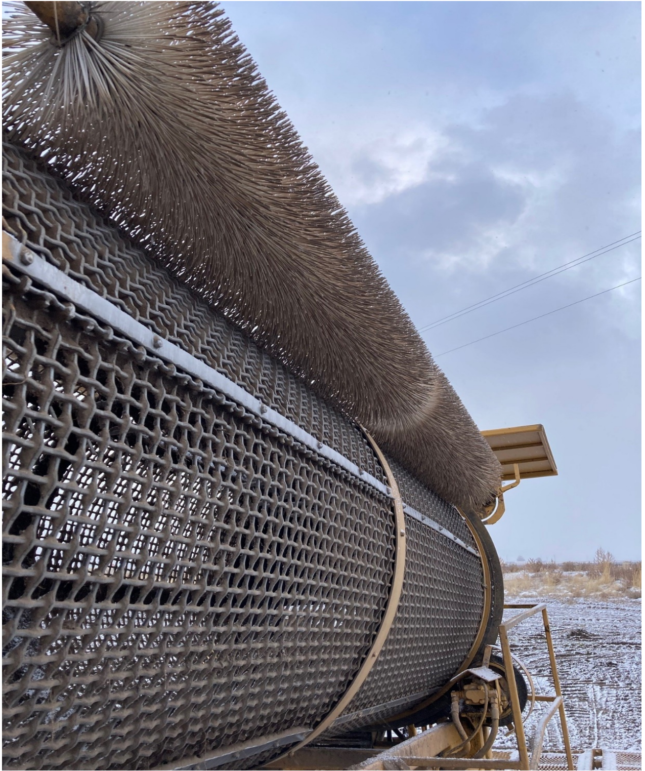
The spinning cage with a brush removes soil from strawberry plant roots
