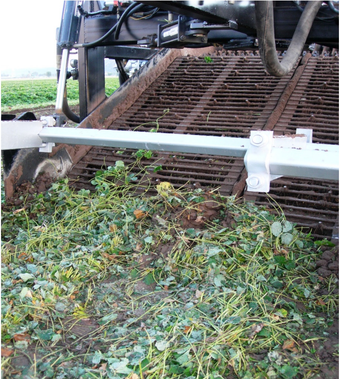
The metal fingers of the digger lift plants to a conveyor
