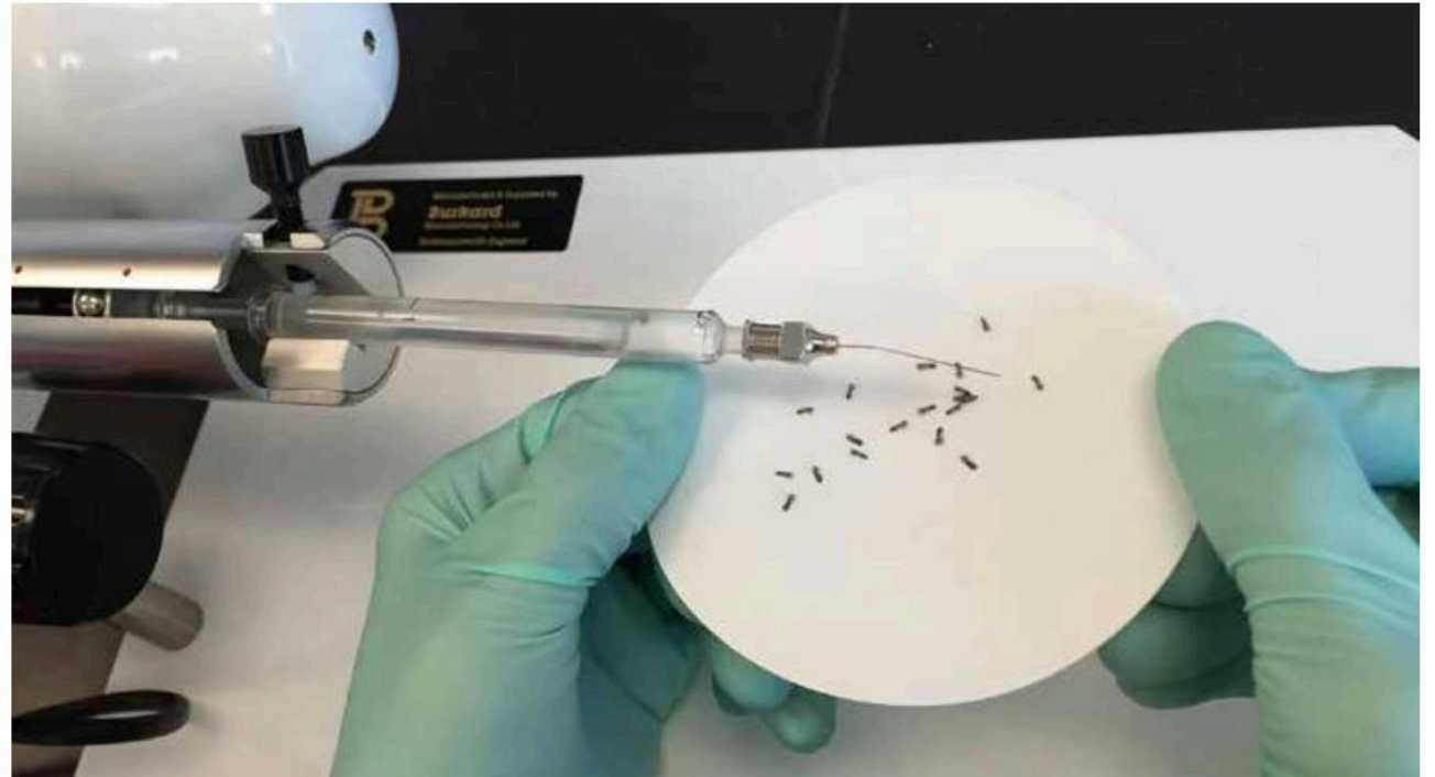
Developing methods for testing pesticide resistance in ACP. We knock them out with CO 2 , apply insecticide on each individual, then conduct a mortality assay.
