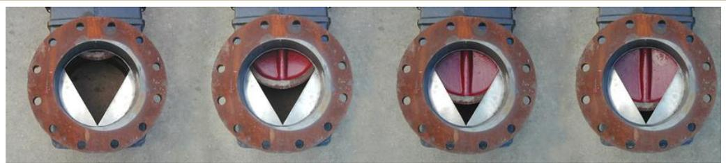
A V-notch gate valve maintains a relatively large opening for solids to pass through even when it is nearly closed, and it also makes it easier to make adjustments at lower flow rates.
