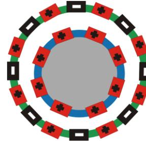
A motor works by lining up the positive charges on the interior shaft with positive charges on the surrounding stationary coil. The like charges repulse, moving the shaft so that it lines up with opposite charges.
