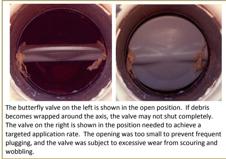
In our experience, a ratchet style controller on a butterfly valve does not give nearly enough flexibility in adjusting flow rates for nutrient application. If using a butterfly valve, an infinitely variable wheel type controller is strongly recommended.
