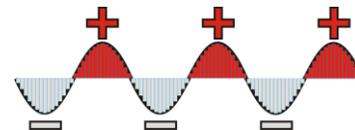
A VFD generates signals that mimic the fluctuations of alternating current (AC) electricity.
