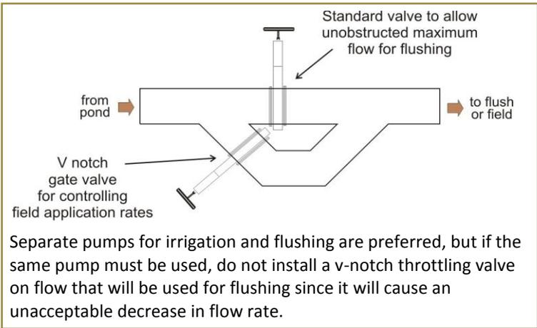
Separate pumps for irrigation and flushing are preferred, but if the same pump must be used, do not install a v-notch throttling valve on flow that will be used for flushing since it will cause an unacceptable decrease in flow rate.
