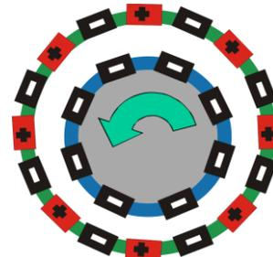
When the polarity changes, the charges become the same, so the shaft has to move again. The speed of the rotation is determined by how quickly the current alternates in polarity.
