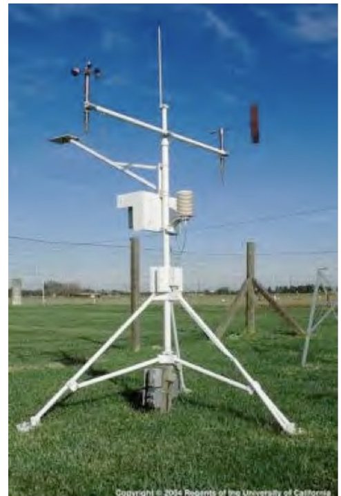
Stations like this measure weather—current conditions like rainfall and windspeed. Climate is the pattern of weather conditions averaged over a very long period of time.
