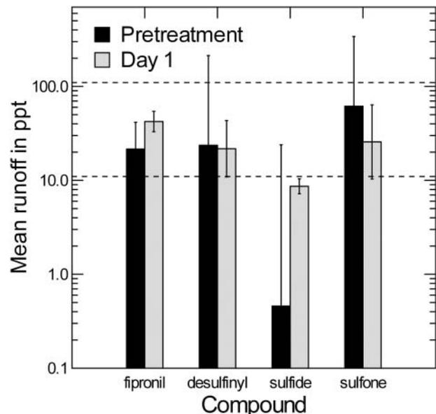
**Figure 5.** Runoff of fipronil and its degradates from four houses treated with a  $2.54 \times 2.54$  cm band (pin stream) in 2013. Upper dashed line is the acute aquatic benchmark (110 ppt) for invertebrates while the lower dashed line is the chronic aquatic benchmark (11 ppt).
