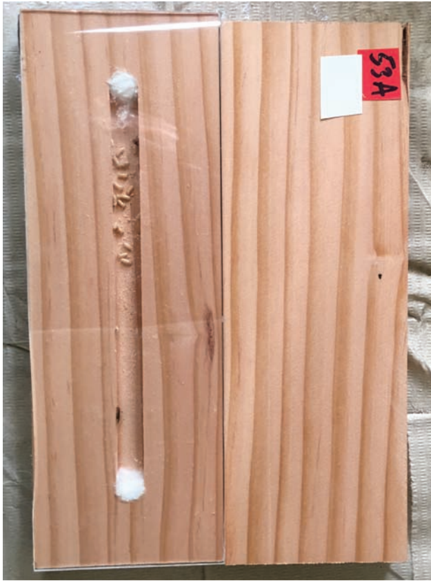
Fig. 1. Disassembled block showing the top (right) and bottom (left) pieces of block. A sheet of acrylic, the cotton balls, and termites inside the channel are shown on the bottom piece of the block (left).
