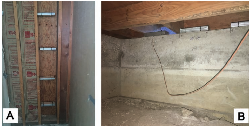
Fig. 3. Two different locations where the experimental blocks were placed. (A) Wall void. Brackets were used to place multiple blocks within a single wall void space. Four blocks are shown in the photo, and the bottommost one is a temperature monitoring block. (B) Subarea. The blocks were placed on the top of concrete perimeter wall. The leftmost block is a temperature monitoring block.
