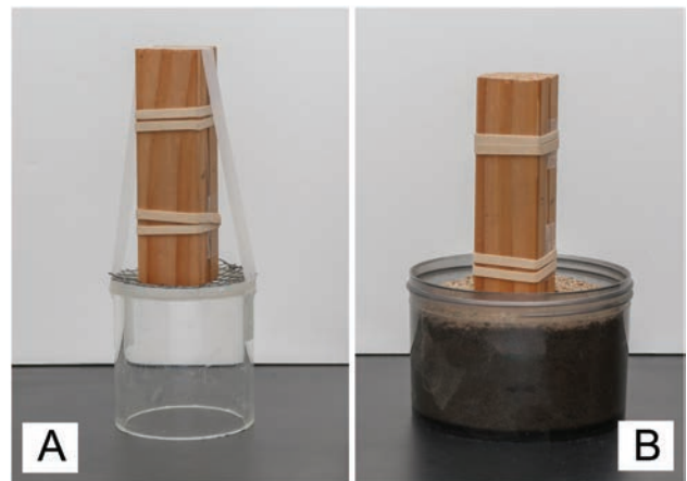
Fig. 3. Arena setups for each trial type. (A) An arena resting on wire mesh on top of a glass cylinder for heat only trials. (B) An arena seated in 600 g of sand for all trials utilizing a heat sink.
