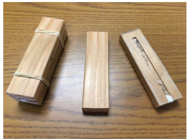
Fig. 2. One assembled arena (left) and disassembled component pieces.
