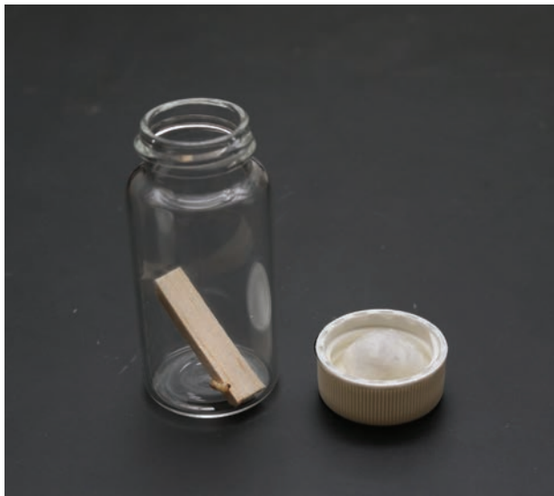
Fig. 1. One vial ready for use in the fumigant toxicity test, including balsa wood, one termite, and cotton inside the cap.
